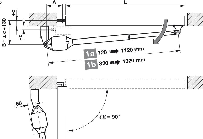
**1a** $L = 1000 \rightarrow 2500 \text{ mm}$ ,  $c = -30 \rightarrow +150 \text{ mm}$
